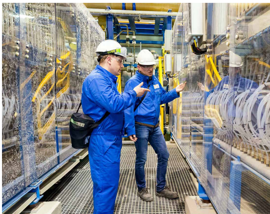
Membrane electrolysis plant of the Chlorine business unit of PCC Rokita SA at our Polish production site in Brzeg Dolny: Early on, in 2015, we completely switched over our chlorine production process to the environmentally compatible and energy-saving membrane technology that is now binding in the EU.
